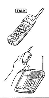
When the headset is connected to the handset (p. 14), be sure to use the headset to talk with the caller. If you want to have a normal corders phone conversation, disconnect the headset.
