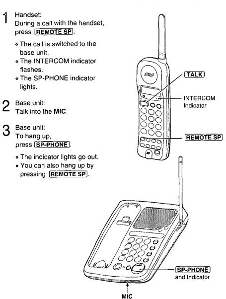
When using the **REDIAL/PAUSE** or **REDIAL** buttons, dialing a stored number (p. 25), etc., press **REMOTE SP** after dialing is completed.
